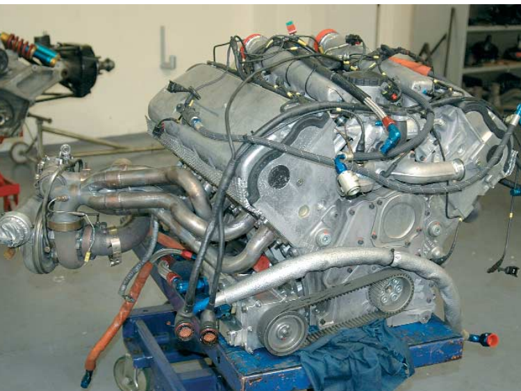
Post-Le Mans and the diesel engine is being prepared for its next race.
