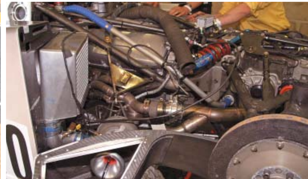
Surprisingly little re-engineering was needed to fit the diesel-fuelled 5.0-litre Volkswagen V10 in place of the petrol-powered Judd V10. A new slimline sump solved the biggest headache of crank-axis height
