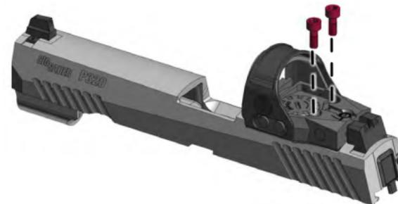
2. Remove the ROMEO from the slide and pull it out of the shroud (if equipped).
