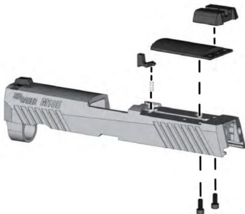
4. Insert the striker assembly into the rear of the slide.
