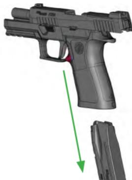
3. Insert a loaded magazine, making sure it is locked into the grip module.
