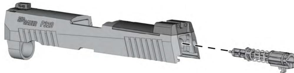
5. Insert the extractor into the right side of the slide.
